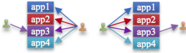
Fig. 6. Reachability: (left) in proactive presence, receiver publishes presence in apps, and the caller knows which to use before a call attempt, vs. (right) caller tries the apps on demand during call-setup until picked by the receiver.
