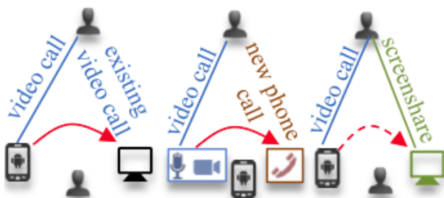
Fig. 4. Call handoff: (a) from one device to another, (b) from one app to another, and (c) call component handoff, e.g., for screenshare.
