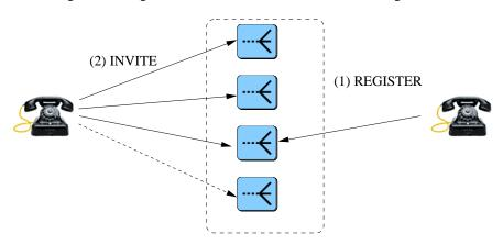
Figure 4: Design B: search for the server on call setup
