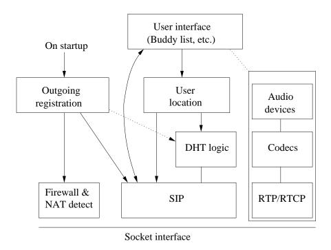
Figure 10: Block diagram of a P2P-SIP node
