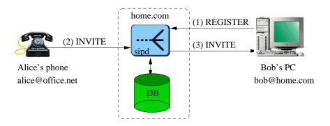
Figure 2: SIP call flow using proxy servers
