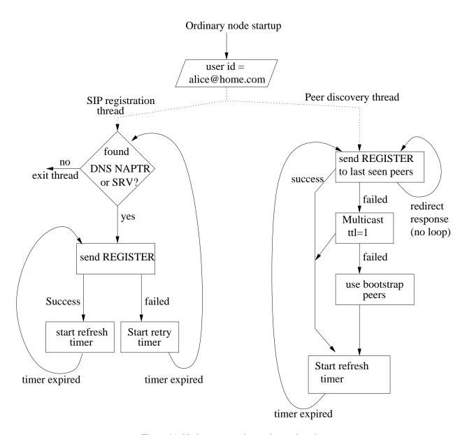
Figure 11: Node startup and outgoing registration
