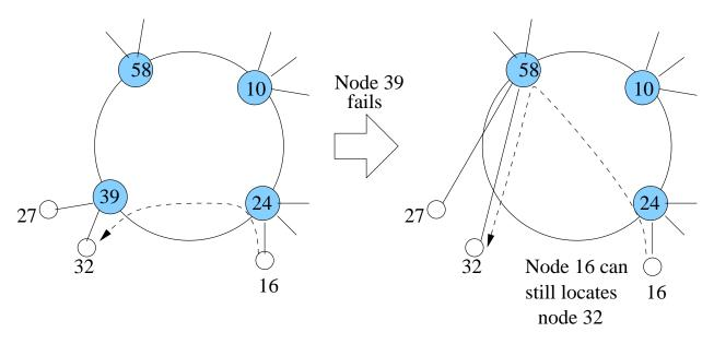
Figure 13: Failure of a super-node in the DHT
